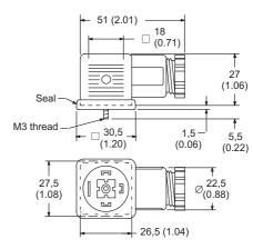
Conductor cross-sectional area: 0,5 to 1,5 mm<sup>2</sup> (0.0008 to 0.0023 in<sup>2</sup>) Cable diameter: 6 to 10 mm (0.24 to 0.40 in)
