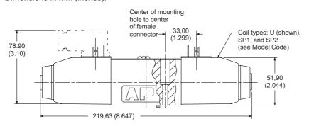
Plug connector can be positioned in 90° increments on valve by removing connector housing and re-assembling contact holder at desired orientation inside housing.
